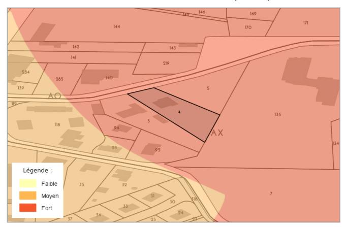
**CARTOGRAPHIE DES MOUVEMENTS DE TERRAINS (ARGILES) - AX3**
