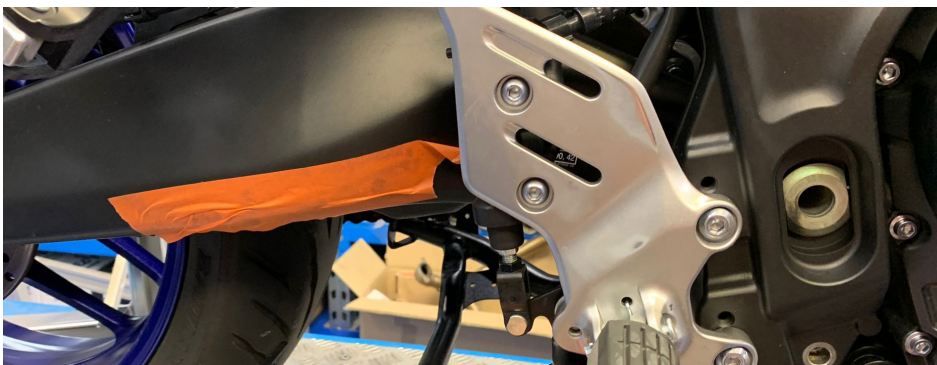
PHOTO 11b - Protect the swingarm with adhesive tape
