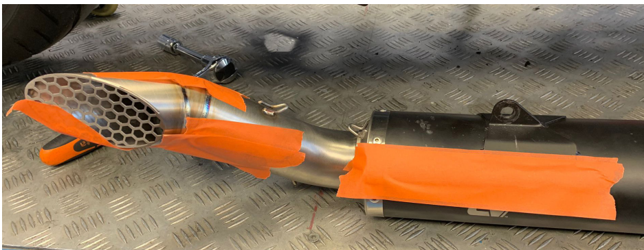
PHOTO 11b - Protect the swingarm with adhesive tape
