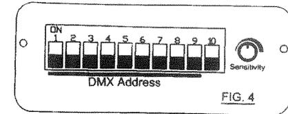
When you set the Dip switches # 10 to "off", one or a few of the other dip switches is(are) on, the unit step into DMX model. Dips 1~9 set the DMX addresses. DMX mode have 6 Chs
